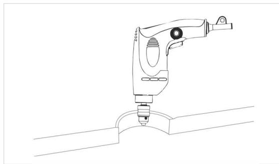
① Drill a hole with Ø60-62mm
